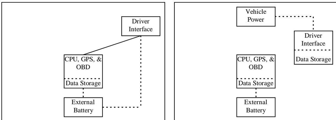
**Figure 5 - Integrated Computer, GPS, and Engine Monitor**
