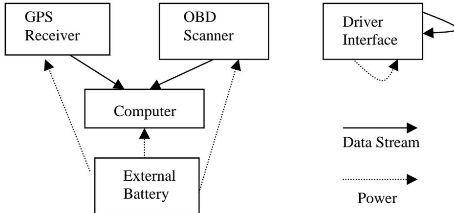
**Figure 6 - Separate Components, Driver Device, and External Battery**
