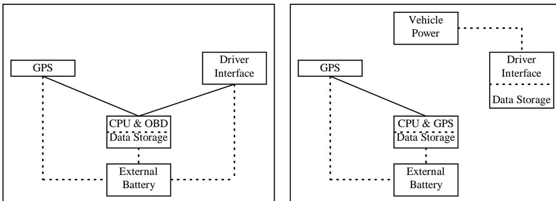
**Figure 3 - Integrated Computer and Engine Monitor**
